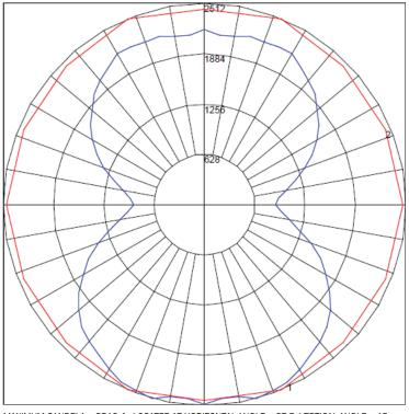
MAXIMUM CANDELA = 2512.4 LOCATED AT HORIZONTAL ANGLE = 67.5, VERTICAL ANGLE = 15 # 1 - VERTICAL PLANE THROUGH HORIZONTAL ANGLES (90 - 270) (THROUGH MAX. CD.) # 2 - HORIZONTAL CONE THROUGH VERTICAL ANGLE (5) (THROUGH MAX. CD.)
