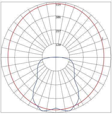
MAXIMUM CANDELA = 514.06 LOCATED AT HORIZONTAL ANGLE = 90, VERTICAL ANGLE = 15 # 1 - VERTICAL PLANE THROUGH HORIZONTAL ANGLES (90 - 270) (THROUGH MAX. CD.) # 2 - HORIZONTAL CONE THROUGH VERTICAL ANGLE (15) (THROUGH MAX. CD.)
