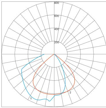
MAXIMUM CANDELA = 751 LOCATED AT HORIZONTAL ANGLE = 0, VERTICAL ANGLE = 19.5 # 1 - VERTICAL PLANE THROUGH HORIZONTAL ANGLES (90 - 270) (THROUGH MAX. CD.) # 2 - VERTICAL PLANE THROUGH HORIZONTAL ANGLES (0 - 180) (THROUGH MAX. CD.)
