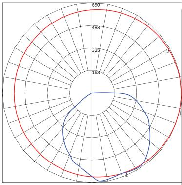
MAXIMUM CANDELA = 650.41 LOCATED AT HORIZONTAL ANGLE = 0, VERTICAL ANGLE = 5 # 1 - VERTICAL PLANE THROUGH HORIZONTAL ANGLES (0 - 180) (THROUGH MAX. CD.) # 2 - HORIZONTAL CONE THROUGH VERTICAL ANGLE (0) (THROUGH MAX. CD.)
