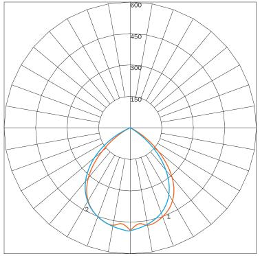
MAXIMUM CANDELA = 504.03 LOCATED AT HORIZONTAL ANGLE = 0, VERTICAL ANGLE = 5 # 1 - VERTICAL PLANE THROUGH HORIZONTAL ANGLES (90 - 270) (THROUGH MAX. CD.) # 2 - VERTICAL PLANE THROUGH HORIZONTAL ANGLES (0 - 180) (THROUGH MAX. CD.)
