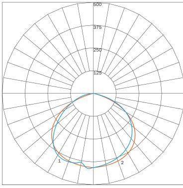
MAXIMUM CANDELA = 416.037 LOCATED AT HORIZONTAL ANGLE = 7, VERTICAL ANGLE = 3 # 1 - VERTICAL PLANE THROUGH HORIZONTAL ANGLES (90 - 270) # 2 - VERTICAL PLANE THROUGH HORIZONTAL ANGLES (0 - 180)
