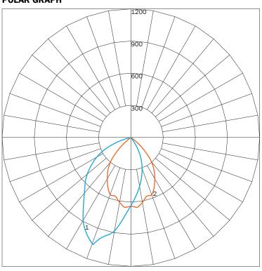
MAXIMUM CANDELA = 1058.53 LOCATED AT HORIZONTAL ANGLE = 0, VERTICAL ANGLE = 19.5 # 1 - VERTICAL PLANE THROUGH HORIZONTAL ANGLES (90 - 270) (THROUGH MAX. CD.) # 2 - VERTICAL PLANE THROUGH HORIZONTAL ANGLES (0 - 180) (THROUGH MAX. CD.)
