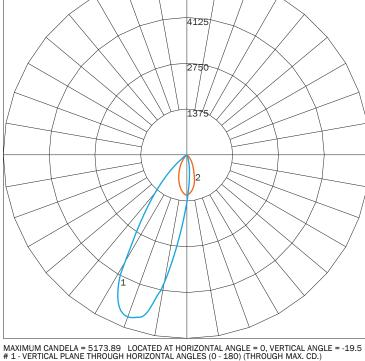
MAXIMUM CANDELA = 5173.89 LOCATED AT HORIZONTAL ANGLE = 0, VERTICAL ANGLE = -19.5 # 1 - VERTICAL PLANE THROUGH HORIZONTAL ANGLES (0 - 180) (THROUGH MAX. CD.) # 2 - HORIZONTAL CONE THROUGH VERTICAL ANGLE (5) (THROUGH MAX. CD.)
