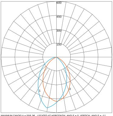
MAXIMUM CANDELA = 556.36 LOCATED AT HORIZONTAL ANGLE = 0, VERTICAL ANGLE = -11 # 1 - VERTICAL PLANE THROUGH HORIZONTAL ANGLES (0 - 180) (THROUGH MAX. CD.) # 2 - HORIZONTAL CONE THROUGH VERTICAL ANGLE (15) (THROUGH MAX. CD.)
