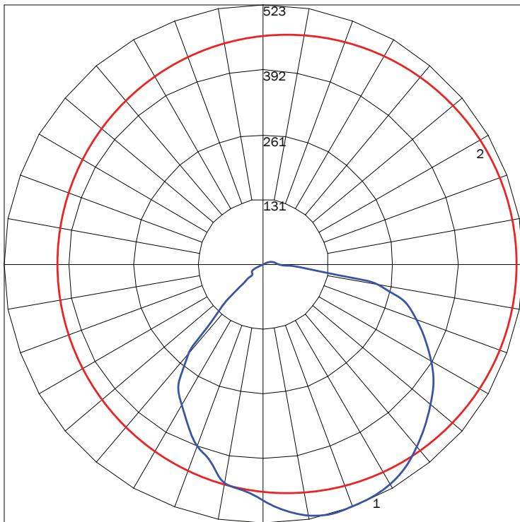
MAXIMUM CANDELA = 522.55 LOCATED AT HORIZONTAL ANGLE = 0, VERTICAL ANGLE = 15
