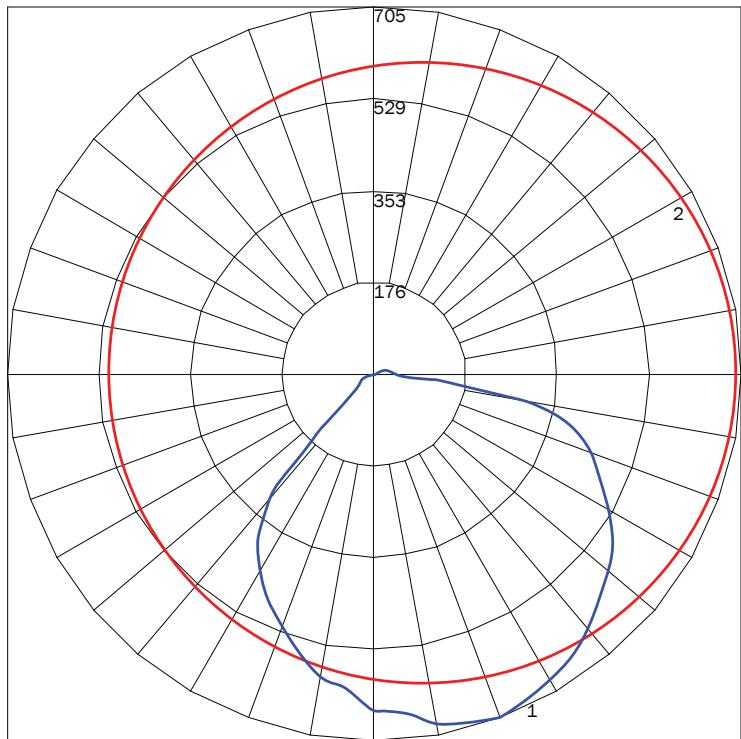
MAXIMUM CANDELA = 705.18 LOCATED AT HORIZONTAL ANGLE = 0, VERTICAL ANGLE = 20
