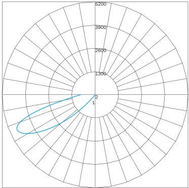
MAXIMUM CANDELA = 5129.88 LOCATED AT HORIZONTAL ANGLE = 0, VERTICAL ANGLE = -65 # 1 - VERTICAL PLANE THROUGH HORIZONTAL ANGLES (90 - 270) (THROUGH MAX. CD.) # 2 - HORIZONTAL CONE THROUGH VERTICAL ANGLE (15) (THROUGH MAX. CD.)
