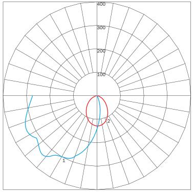
MAXIMUM CANDELA = 346.617 LOCATED AT HORIZONTAL ANGLE = 0, VERTICAL ANGLE = -42.5 # 1 - VERTICAL PLANE THROUGH HORIZONTAL ANGLES (90 - 270) (THROUGH MAX. CD.) # 2 - HORIZONTAL CONE THROUGH VERTICAL ANGLE (15) (THROUGH MAX. CD.)
