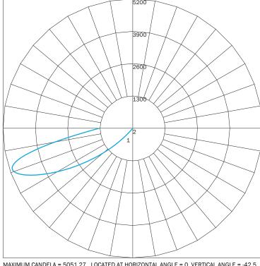
MAXIMUM CANDELA = 5051.27 LOCATED AT HORIZONTAL ANGLE = 0, VERTICAL ANGLE = -42.5 # 1 - VERTICAL PLANE THROUGH HORIZONTAL ANGLES (0 - 180) (THROUGH MAX. CD.) # 2 - HORIZONTAL CONE THROUGH VERTICAL ANGLE (5) (THROUGH MAX. CD.)
