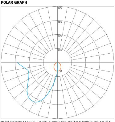
MAXIMUM CANDELA = 491.21 LOCATED AT HORIZONTAL ANGLE = -5, VERTICAL ANGLE = -37.5 # 1 - VERTICAL PLANE THROUGH HORIZONTAL ANGLES (15 - 195) (THROUGH MAX. CD.) # 2 - HORIZONTAL CONE THROUGH VERTICAL ANGLE (10) (THROUGH MAX. CD.)
