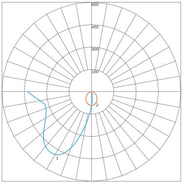
MAXIMUM CANDELA = 491.21 LOCATED AT HORIZONTAL ANGLE = -5, VERTICAL ANGLE = -37.5 # 1 - VERTICAL PLANE THROUGH HORIZONTAL ANGLES (15 - 195) (THROUGH MAX. CD.) # 2 - HORIZONTAL CONE THROUGH VERTICAL ANGLE (10) (THROUGH MAX. CD.)
