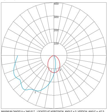
MAXIMUM CANDELA = 346.617 LOCATED AT HORIZONTAL ANGLE = 0, VERTICAL ANGLE = -42.5 # 1 - VERTICAL PLANE THROUGH HORIZONTAL ANGLES (90 - 270) (THROUGH MAX. CD.) # 2 - HORIZONTAL CONE THROUGH VERTICAL ANGLE (15) (THROUGH MAX. CD.)
