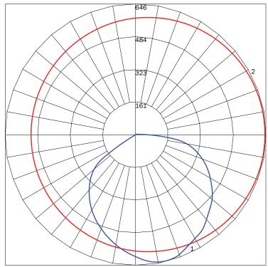
MAXIMUM CANDELA = 645.67 LOCATED AT HORIZONTAL ANGLE = 45, VERTICAL ANGLE = 15 # 1 - VERTICAL PLANE THROUGH HORIZONTAL ANGLES (45 - 225) (THROUGH MAX. CD.) # 2 - HORIZONTAL CONE THROUGH VERTICAL ANGLE (15) (THROUGH MAX. CD.)
