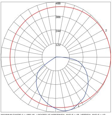
MAXIMUM CANDELA = 488.16 LOCATED AT HORIZONTAL ANGLE = 45, VERTICAL ANGLE = 10 # 1 - VERTICAL PLANE THROUGH HORIZONTAL ANGLES (45 - 225) (THROUGH MAX. CD.) # 2 - HORIZONTAL CONE THROUGH VERTICAL ANGLE (10) (THROUGH MAX. CD.)
