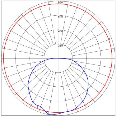
MAXIMUM CANDELA = 859.72 LOCATED AT HORIZONTAL ANGLE = 180, VERTICAL ANGLE = 10 # 1 - VERTICAL PLANE THROUGH HORIZONTAL ANGLES (0 - 180) (THROUGH MAX. CD.) # 2 - HORIZONTAL CONE THROUGH VERTICAL ANGLE (10) (THROUGH MAX. CD.)
