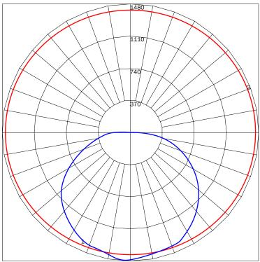
MAXIMUM CANDELA = 2479.53 LOCATED AT HORIZONTAL ANGLE = 157.5, VERTICAL ANGLE = 5 # 1 - VERTICAL PLANE THROUGH HORIZONTAL ANGLES (157.5 - 337.5) (THROUGH MAX. CD.) # 2 - HORIZONTAL CONE THROUGH VERTICAL ANGLE (5) (THROUGH MAX. CD.)
