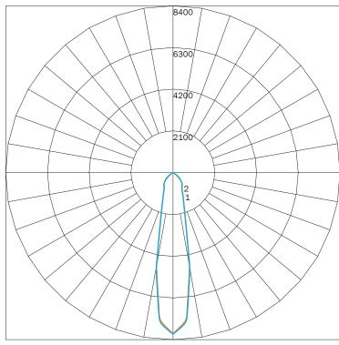
MAXIMUM CANDELA = 8126.01 LOCATED AT HORIZONTAL ANGLE = 0, VERTICAL ANGLE = 0 # 1 - VERTICAL PLANE THROUGH HORIZONTAL ANGLES (90 - 270) # 2 - VERTICAL PLANE THROUGH HORIZONTAL ANGLES (0 - 180)
