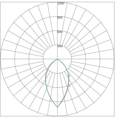
MAXIMUM CANDELA = 1010.88 LOCATED AT HORIZONTAL ANGLE = 0, VERTICAL ANGLE = 0 # 1 - VERTICAL PLANE THROUGH HORIZONTAL ANGLES (90 - 270) # 2 - VERTICAL PLANE THROUGH HORIZONTAL ANGLES (0 - 180)
