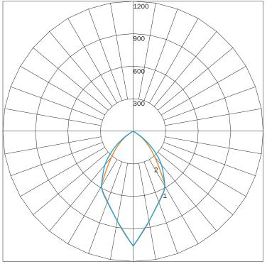
MAXIMUM CANDELA = 1058.22 LOCATED AT HORIZONTAL ANGLE = 0, VERTICAL ANGLE = 0 # 1 - VERTICAL PLANE THROUGH HORIZONTAL ANGLES (90 - 270) # 2 - VERTICAL PLANE THROUGH HORIZONTAL ANGLES (0 - 180)
