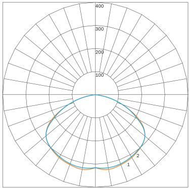
MAXIMUM CANDELA = 342.405 LOCATED AT HORIZONTAL ANGLE = 180, VERTICAL ANGLE = 5 # 1 - VERTICAL PLANE THROUGH HORIZONTAL ANGLES (0 - 180) # 2 - VERTICAL PLANE THROUGH HORIZONTAL ANGLES (90 - 270)
