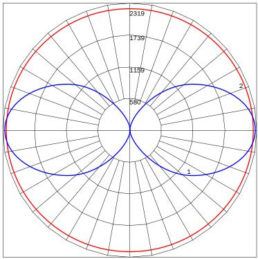
MAXIMUM CANDELA = 2318.86 LOCATED AT HORIZONTAL ANGLE = 45, VERTICAL ANGLE = 90 # 1 - VERTICAL PLANE THROUGH HORIZONTAL ANGLES (45 - 225) (THROUGH MAX. CD.) # 2 - HORIZONTAL CONE THROUGH VERTICAL ANGLE (90) (THROUGH MAX. CD.)
