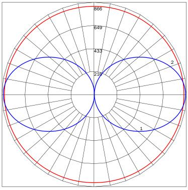
MAXIMUM CANDELA = 865.78 LOCATED AT HORIZONTAL ANGLE = 67.5, VERTICAL ANGLE = 90 # 1 - VERTICAL PLANE THROUGH HORIZONTAL ANGLES (67.5 - 247.5) (THROUGH MAX. CD.) # 2 - HORIZONTAL CONE THROUGH VERTICAL ANGLE (90) (THROUGH MAX. CD.)
