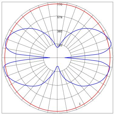
MAXIMUM CANDELA = 2962.16 LOCATED AT HORIZONTAL ANGLE = 157.5, VERTICAL ANGLE = 5 # 1 - VERTICAL PLANE THROUGH HORIZONTAL ANGLES (157.5 - 337.5) (THROUGH MAX. CD.) # 2 - HORIZONTAL CONE THROUGH VERTICAL ANGLE (5) (THROUGH MAX. CD.)
