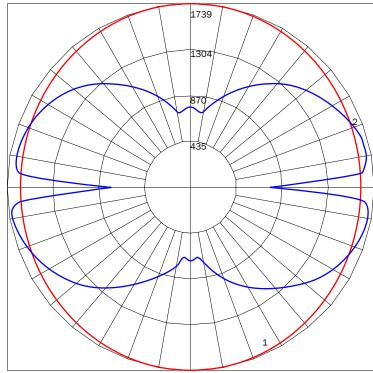
MAXIMUM CANDELA = 3017.67 LOCATED AT HORIZONTAL ANGLE = 0, VERTICAL ANGLE = 10 # 1 - VERTICAL PLANE THROUGH HORIZONTAL ANGLES (0 - 180) (THROUGH MAX. CD.) # 2 - HORIZONTAL CONE THROUGH VERTICAL ANGLE (10) (THROUGH MAX. CD.)
