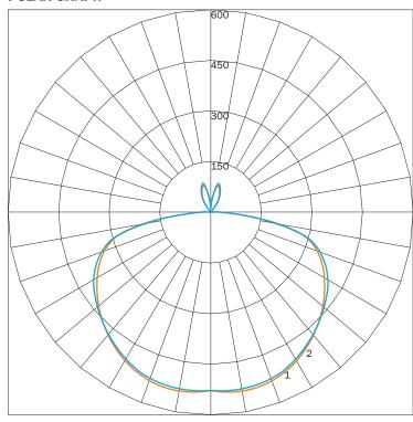
MAXIMUM CANDELA = 576.011 LOCATED AT HORIZONTAL ANGLE = 67.5, VERTICAL ANGLE = 5 # 1 - VERTICAL PLANE THROUGH HORIZONTAL ANGLES (90 - 270) # 2 - VERTICAL PLANE THROUGH HORIZONTAL ANGLES (0 - 180)
