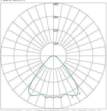
MAXIMUM CANDELA = 420.9 LOCATED AT HORIZONTAL ANGLE = 150, VERTICAL ANGLE = 30 # 1 - VERTICAL PLANE THROUGH HORIZONTAL ANGLES (90 - 270) # 2 - VERTICAL PLANE THROUGH HORIZONTAL ANGLES (0 - 180)
