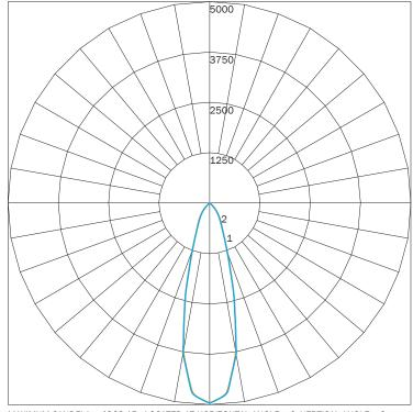
MAXIMUM CANDELA = 4966.15 LOCATED AT HORIZONTAL ANGLE = 0, VERTICAL ANGLE = 0 # 1 - VERTICAL PLANE THROUGH HORIZONTAL ANGLES (90 - 270) # 2 - VERTICAL PLANE THROUGH HORIZONTAL ANGLES (0 - 180)
