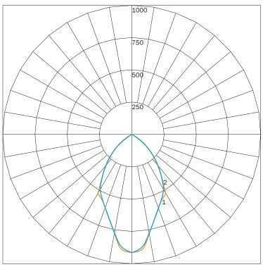
MAXIMUM CANDELA = 913.88 LOCATED AT HORIZONTAL ANGLE = 0, VERTICAL ANGLE = 0 # 1 - VERTICAL PLANE THROUGH HORIZONTAL ANGLES (90 - 270) # 2 - VERTICAL PLANE THROUGH HORIZONTAL ANGLES (0 - 180)
