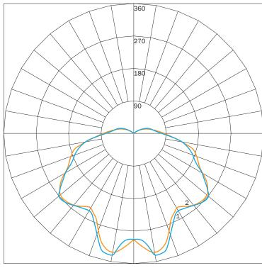
MAXIMUM CANDELA = 341.72 LOCATED AT HORIZONTAL ANGLE = 180, VERTICAL ANGLE = 5 # 1 - VERTICAL PLANE THROUGH HORIZONTAL ANGLES (90 - 270) # 2 - VERTICAL PLANE THROUGH HORIZONTAL ANGLES (0 - 180)
