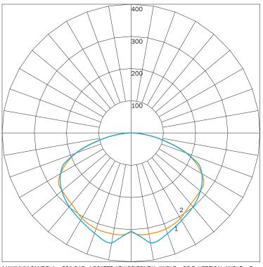
MAXIMUM CANDELA = 351.915 LOCATED AT HORIZONTAL ANGLE = 22.5, VERTICAL ANGLE = 5 # 1 - VERTICAL PLANE THROUGH HORIZONTAL ANGLES (90 - 270) # 2 - VERTICAL PLANE THROUGH HORIZONTAL ANGLES (0 - 180)
