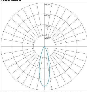
MAXIMUM CANDELA =  $5102.8\,$  LOCATED AT HORIZONTAL ANGLE = 0, VERTICAL ANGLE = 0 # 1 - VERTICAL PLANE THROUGH HORIZONTAL ANGLES (90 - 270) # 2 - VERTICAL PLANE THROUGH HORIZONTAL ANGLES (0 - 180)
