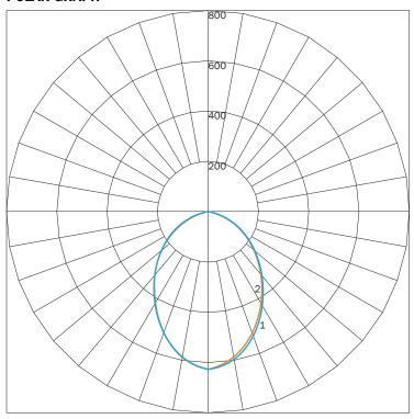
MAXIMUM CANDELA = 637.69 LOCATED AT HORIZONTAL ANGLE = 60, VERTICAL ANGLE = 5 # 1 - VERTICAL PLANE THROUGH HORIZONTAL ANGLES (90 - 270) # 2 - VERTICAL PLANE THROUGH HORIZONTAL ANGLES (0 - 180)
