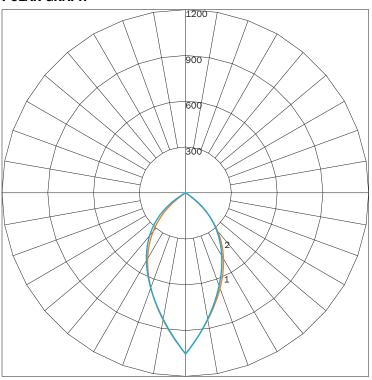
MAXIMUM CANDELA = 1053.46 LOCATED AT HORIZONTAL ANGLE = 0, VERTICAL ANGLE = 0 # 1 - VERTICAL PLANE THROUGH HORIZONTAL ANGLES (90 - 270) # 2 - VERTICAL PLANE THROUGH HORIZONTAL ANGLES (0 - 180)
