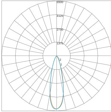
MAXIMUM CANDELA = 5300.68 LOCATED AT HORIZONTAL ANGLE = 0, VERTICAL ANGLE = 0 # 1 - VERTICAL PLANE THROUGH HORIZONTAL ANGLES (90 - 270) # 2 - VERTICAL PLANE THROUGH HORIZONTAL ANGLES (0 - 180)
