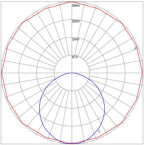
MAXIMUM CANDELA = 3893.9 LOCATED AT HORIZONTAL ANGLE = 90, VERTICAL ANGLE = 5 # 1 - VERTICAL PLANE THROUGH HORIZONTAL ANGLES (90 - 270) (THROUGH MAX. CD.) # 2 - HORIZONTAL CONE THROUGH VERTICAL ANGLE (5) (THROUGH MAX. CD.)
