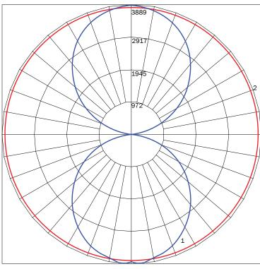
MAXIMUM CANDELA = 3899.18 LOCATED AT HORIZONTAL ANGLE = 67.5, VERTICAL ANGLE = 5 # 1 - VERTICAL PLANE THROUGH HORIZONTAL ANGLES (65.7 - 247.5) (THROUGH MAX. CD.) # 2 - HORIZONTAL CONE THROUGH VERTICAL ANGLE (5) (THROUGH MAX. CD.)
