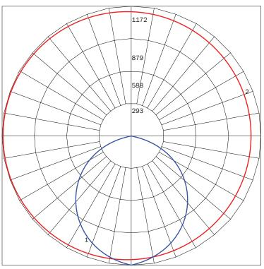
MAXIMUM CANDELA = 1172.49 LOCATED AT HORIZONTAL ANGLE = 0, VERTICAL ANGLE = 0 # 1 - VERTICAL PLANE THROUGH HORIZONTAL ANGLES (0 - 180) (THROUGH MAX. CD) # 2 - HORIZONTAL CONE THROUGH VERTICAL ANGLE (0) (THROUGH MAX. CD)
