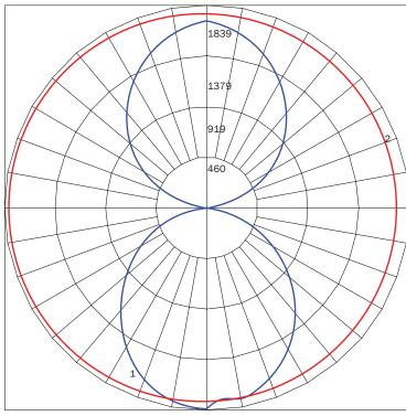
MAXIMUM CANDELA = 1838.81 LOCATED AT HORIZONTAL ANGLE = 180, VERTICAL ANGLE = 5 # 1 - VERTICAL PLANE THROUGH HORIZONTAL ANGLES (180 - 0) (THROUGH MAX. CD) # 2 - HORIZONTAL CONE THROUGH VERTICAL ANGLE (5) (THROUGH MAX. CD)
