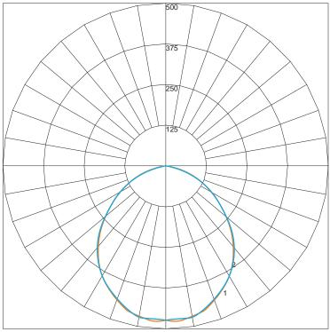
MAXIMUM CANDELA = 487.35 LOCATED AT HORIZONTAL ANGLE = 45, VERTICAL ANGLE = 5 # 1 - VERTICAL PLANE THROUGH HORIZONTAL ANGLES (90 - 270) # 2 - VERTICAL PLANE THROUGH HORIZONTAL ANGLES (0 - 180)
