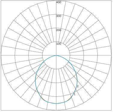
MAXIMUM CANDELA = 353.99 LOCATED AT HORIZONTAL ANGLE = 0, VERTICAL ANGLE = 5 # 1 - VERTICAL PLANE THROUGH HORIZONTAL ANGLES (90 - 270) # 2 - VERTICAL PLANE THROUGH HORIZONTAL ANGLES (0 - 180)
