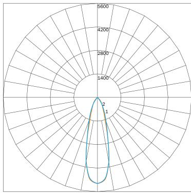
MAXIMUM CANDELA = 5115.48 LOCATED AT HORIZONTAL ANGLE = 0, VERTICAL ANGLE = 0 # 1 - VERTICAL PLANE THROUGH HORIZONTAL ANGLES (90 - 270) # 2 - VERTICAL PLANE THROUGH HORIZONTAL ANGLES (0 - 180)
