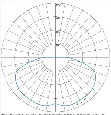
MAXIMUM CANDELA = 274.644 LOCATED AT HORIZONTAL ANGLE = 0, VERTICAL ANGLE = 15 # 1 - VERTICAL PLANE THROUGH HORIZONTAL ANGLES (90 - 270) # 2 - VERTICAL PLANE THROUGH HORIZONTAL ANGLES (0 - 180)
