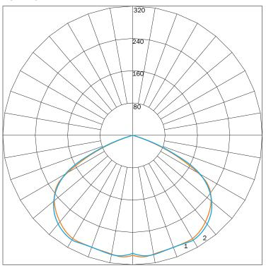
MAXIMUM CANDELA = 309.726 LOCATED AT HORIZONTAL ANGLE = 90, VERTICAL ANGLE = 5 # 1 - VERTICAL PLANE THROUGH HORIZONTAL ANGLES (90 - 270) # 2 - VERTICAL PLANE THROUGH HORIZONTAL ANGLES (0 - 180)
