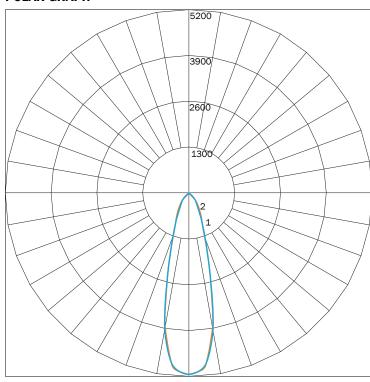
MAXIMUM CANDELA = 51353.46 LOCATED AT HORIZONTAL ANGLE = 0, VERTICAL ANGLE = 0 # 1 - VERTICAL PLANE THROUGH HORIZONTAL ANGLES (90 - 270) # 2 - VERTICAL PLANE THROUGH HORIZONTAL ANGLES (0 - 180)
