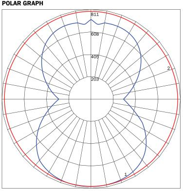
MAXIMUM CANDELA = 810.88 LOCATED AT HORIZONTAL ANGLE = 90, VERTICAL ANGLE = 15 # 1 - VERTICAL PLANE THROUGH HORIZONTAL ANGLES (90 - 270) (THROUGH MAX. CD.) # 2 - HORIZONTAL CONE THROUGH VERTICAL ANGLE (15) (THROUGH MAX. CD.)
