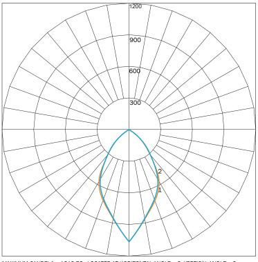
MAXIMUM CANDELA = 1019.78 LOCATED AT HORIZONTAL ANGLE = 0, VERTICAL ANGLE = 0 # 1 - VERTICAL PLANE THROUGH HORIZONTAL ANGLES (90 - 270) # 2 - VERTICAL PLANE THROUGH HORIZONTAL ANGLES (0 - 180)
