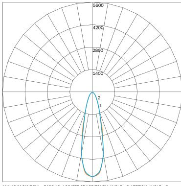
MAXIMUM CANDELA = 5198.16 LOCATED AT HORIZONTAL ANGLE = 0, VERTICAL ANGLE = 0 # 1 - VERTICAL PLANE THROUGH HORIZONTAL ANGLES (90 - 270) # 2 - VERTICAL PLANE THROUGH HORIZONTAL ANGLES (0 - 180)
