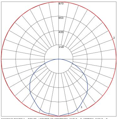
MAXIMUM CANDELA = 870.39 LOCATED AT HORIZONTAL ANGLE = 0, VERTICAL ANGLE = 0 # 1 - VERTICAL PLANE THROUGH HORIZONTAL ANGLES (0 - 180) (THROUGH MAX. CD.) # 2 - HORIZONTAL CONE THROUGH VERTICAL ANGLE (0) (THROUGH MAX. CD.)
