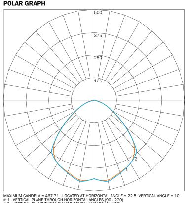
MAXIMUM CANDELA = 467.71 LOCATED AT HORIZONTAL ANGLE = 22.5, VERTICAL ANGLE = 10 # 1 - VERTICAL PLANE THROUGH HORIZONTAL ANGLES (90 - 270) # 2 - VERTICAL PLANE THROUGH HORIZONTAL ANGLES (0 - 180)
