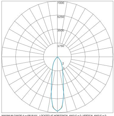
MAXIMUM CANDELA = 6818.64 LOCATED AT HORIZONTAL ANGLE = 0, VERTICAL ANGLE = 0 # 1 - VERTICAL PLANE THROUGH HORIZONTAL ANGLES (90 - 270) # 2 - VERTICAL PLANE THROUGH HORIZONTAL ANGLES (0 - 180)
