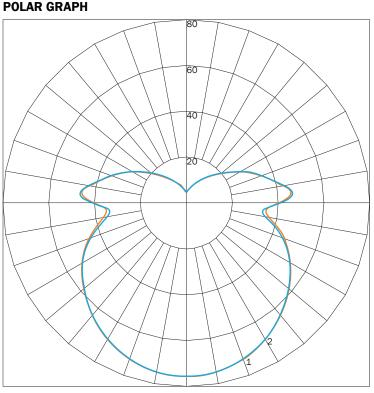
MAXIMUM CANDELA = 75.882 LOCATED AT HORIZONTAL ANGLE = 90, VERTICAL ANGLE = 1 # 1 - VERTICAL PLANE THROUGH HORIZONTAL ANGLES (90 - 270) # 2 - VERTICAL PLANE THROUGH HORIZONTAL ANGLES (0 - 180)
