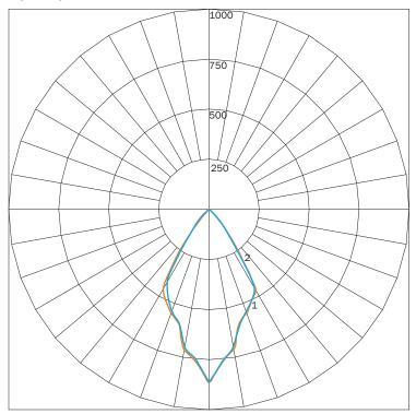
MAXIMUM CANDELA = 862.42 LOCATED AT HORIZONTAL ANGLE = 0, VERTICAL ANGLE = 0 # 1 - VERTICAL PLANE THROUGH HORIZONTAL ANGLES (90 - 270) # 2 - VERTICAL PLANE THROUGH HORIZONTAL ANGLES (0 - 180)
