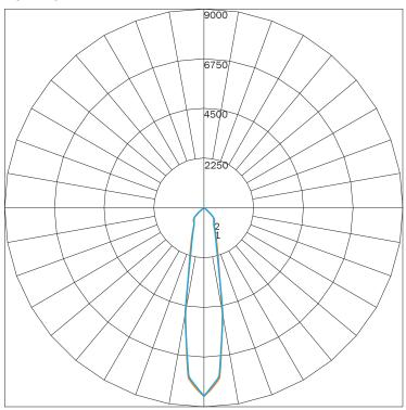
MAXIMUM CANDELA = 8523.55 LOCATED AT HORIZONTAL ANGLE = 0, VERTICAL ANGLE = 0 # 1 - VERTICAL PLANE THROUGH HORIZONTAL ANGLES (90 - 270) # 2 - VERTICAL PLANE THROUGH HORIZONTAL ANGLES (0 - 180)
