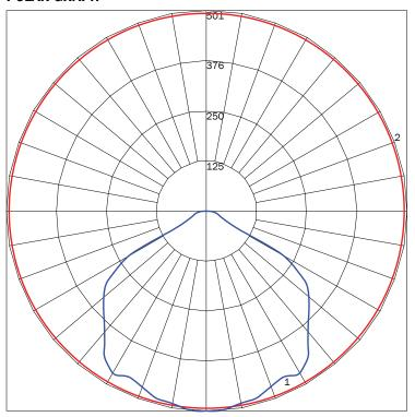
MAXIMUM CANDELA = 500.83 LOCATED AT HORIZONTAL ANGLE = 22.5, VERTICAL ANGLE = 5 # 1 - VERTICAL PLANE THROUGH HORIZONTAL ANGLES (22.5 - 202.5) (THROUGH MAX. CD.) # 2 - HORIZONTAL CONE THROUGH VERTICAL ANGLE (90) (THROUGH MAX. CD.)
