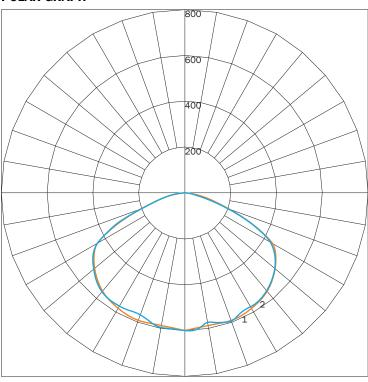
MAXIMUM CANDELA = 604.377 LOCATED AT HORIZONTAL ANGLE = 0, VERTICAL ANGLE = 5 # 1 - VERTICAL PLANE THROUGH HORIZONTAL ANGLES (90 - 270) # 2 - VERTICAL PLANE THROUGH HORIZONTAL ANGLES (0 - 180)
