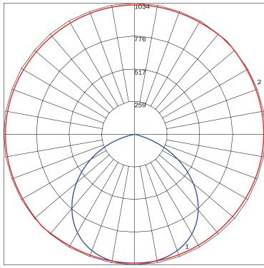
MAXIMUM CANDELA = 1034.22 LOCATED AT HORIZONTAL ANGLE = 0, VERTICAL ANGLE = 0 # 1 - VERTICAL PLANE THROUGH HORIZONTAL ANGLES (0 - 189) (THROUGH MAX. CD.) # 2 - HORIZONTAL CONE THROUGH VERTICAL ANGLE (0) (THROUGH MAX. CD.)
