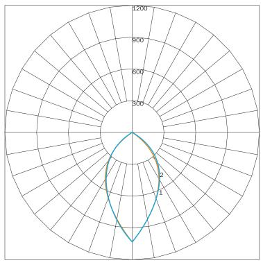
MAXIMUM CANDELA = 1032.22 LOCATED AT HORIZONTAL ANGLE = 0, VERTICAL ANGLE = 0 # 1 - VERTICAL PLANE THROUGH HORIZONTAL ANGLES (90 - 270) # 2 - VERTICAL PLANE THROUGH HORIZONTAL ANGLES (0 - 180)
