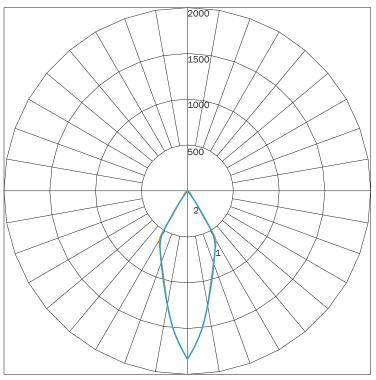
MAXIMUM CANDELA = 1833.69 LOCATED AT HORIZONTAL ANGLE = 0, VERTICAL ANGLE = 0 # 1 - VERTICAL PLANE THROUGH HORIZONTAL ANGLES (90 - 270) # 2 - VERTICAL PLANE THROUGH HORIZONTAL ANGLES (0 - 180)
